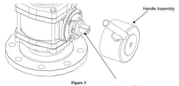
Actuator Shaft If the direction of rotation is to be changed, remove the stop plate from the actuator shaft, rotate 90 degrees with respect to the actuator shaft, then replace the stop plate on the actuator shaft. Then rotate the actuator shaft so that the ball is in the closed position. (See Figure 4)
